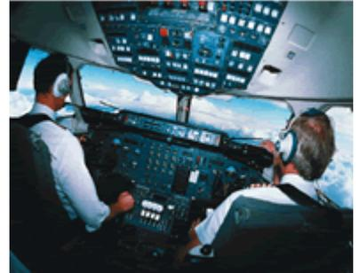
Pilots use the control panels of this passenger aircraft to follow air traffic control commands, to adjust for wind currents, and to avoid the airspace of other planes.
